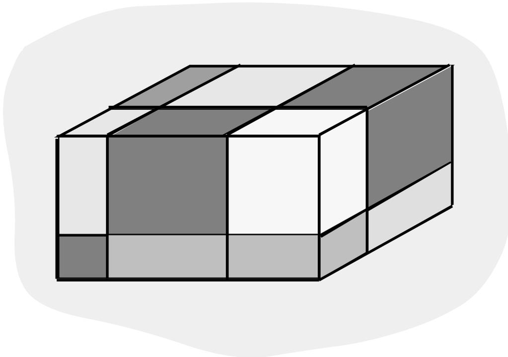
The user simply defines the X, Y and Z mesh boundaries in increasing order and the supplies a material map for the mesh system.
