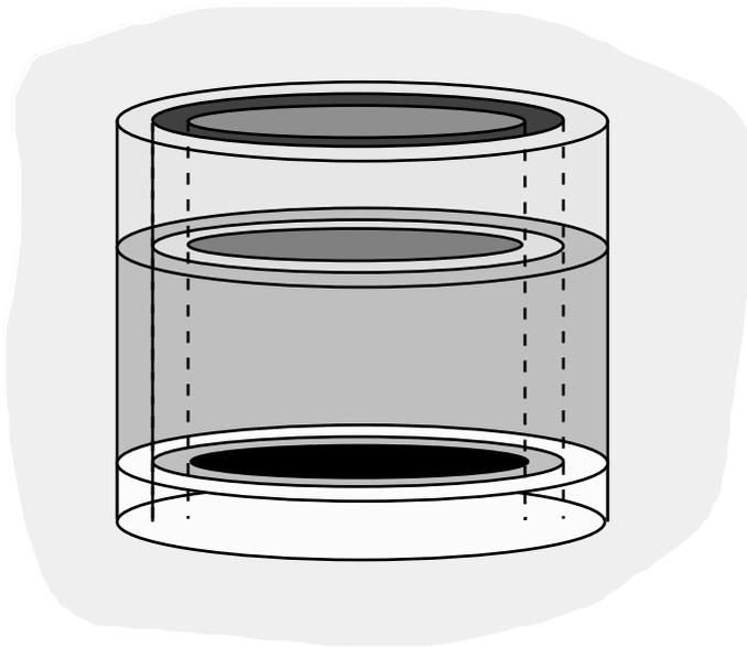
The user simply defines the R and Z mesh boundaries in increasing order and then supplies a material map for the mesh system. A vertical cross-section through the centre of the above mesh system is shown below:
