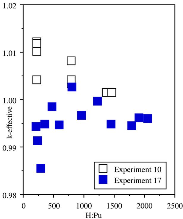
Figure 3 - Calculated k-effective against H:Pu for Mixed Nitrate Solution Experiments
