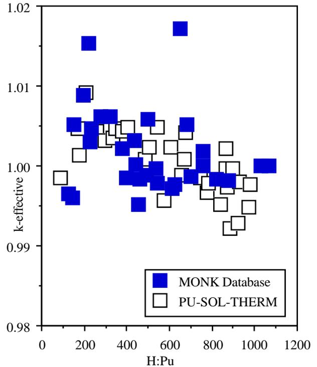
Figure 5 - Calculated k-effective against H:Pu for Plutonium Nitrate Solution Experiments
