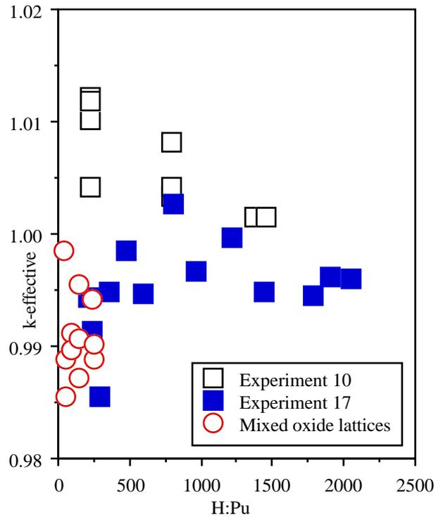
Figure 4 - Calculated k-effective against H:Pu for Mixed Nitrate Solution and Mixed Oxide Experiments
