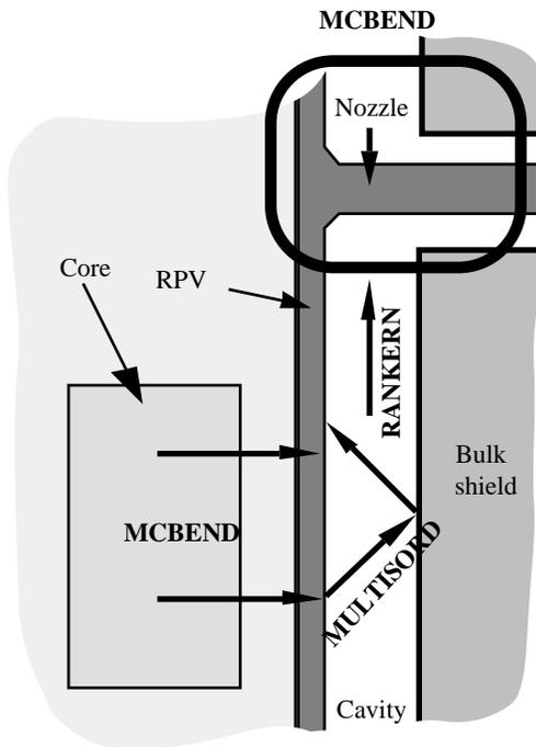
Figure 1 - Calculational route for LWR cavity streaming
