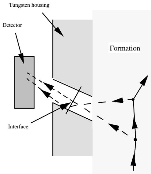
Figure 3 - The Forced Flight Mechanism
