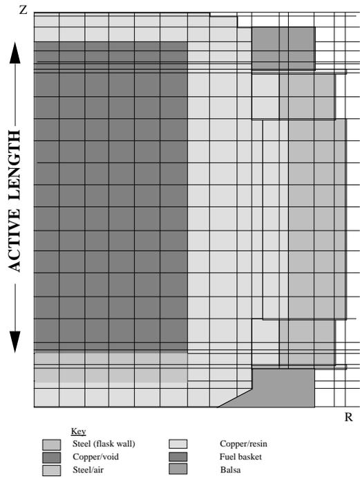
Figure 1 - MAGIC representation of dry fuel transport flask
