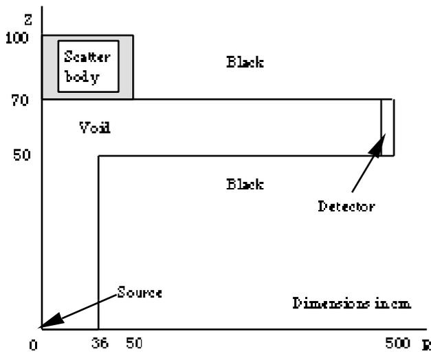
Figure 7 - Test case for angular biasing of scatter
