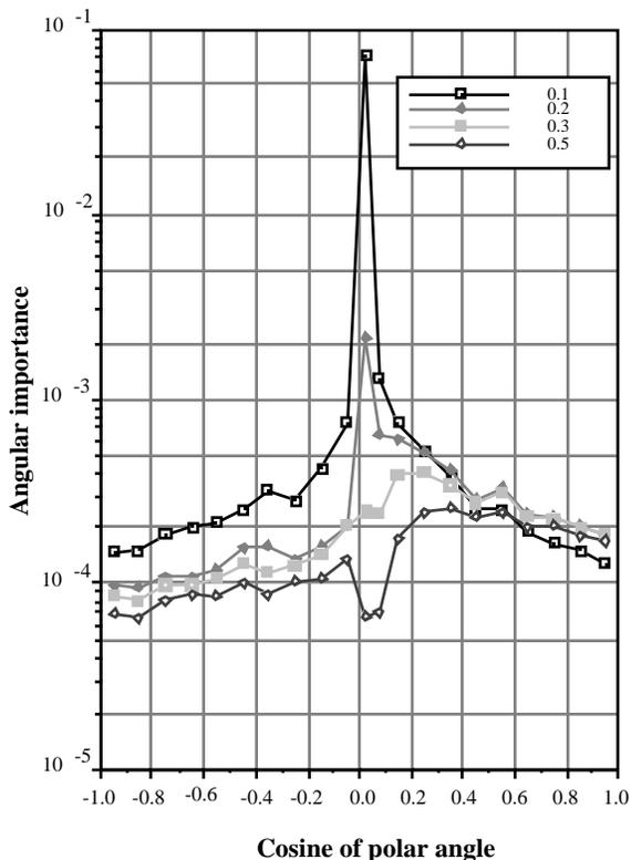
Figure 6 - Variation of angular importances at the edge of a duct
