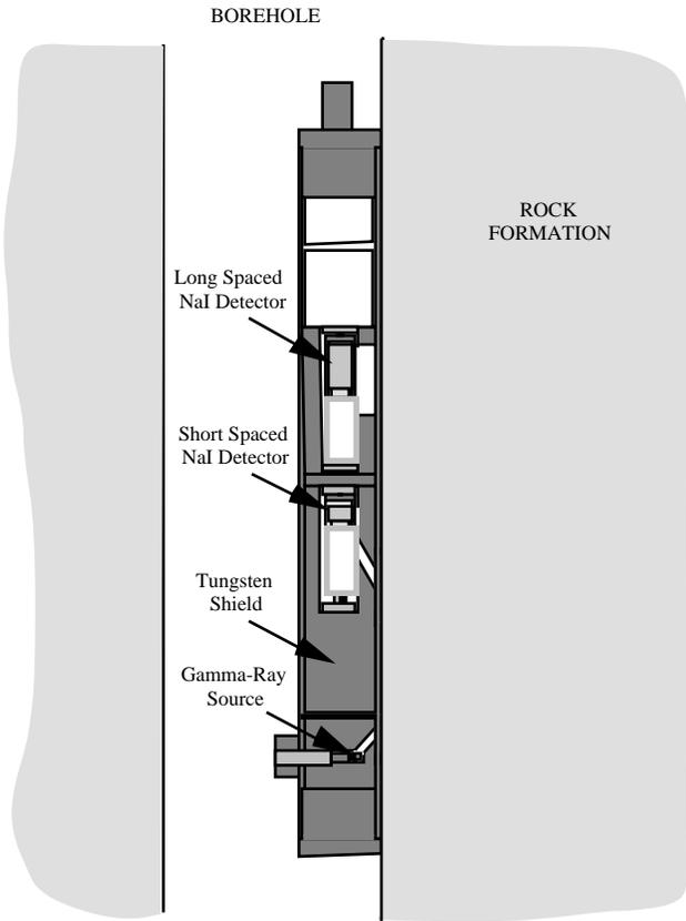
Figure 2 - Gamma-ray Density Sonde
