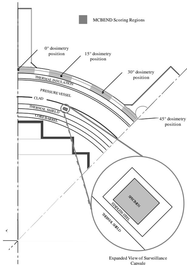
Figure 2. H B Robinson radial shield model
