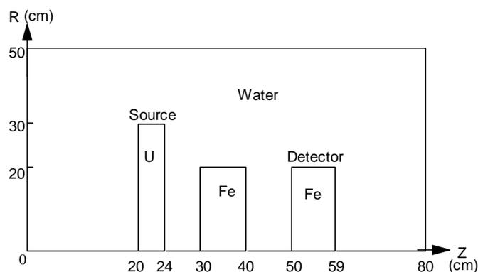
Figure 1. Geometry for Test Case 8
