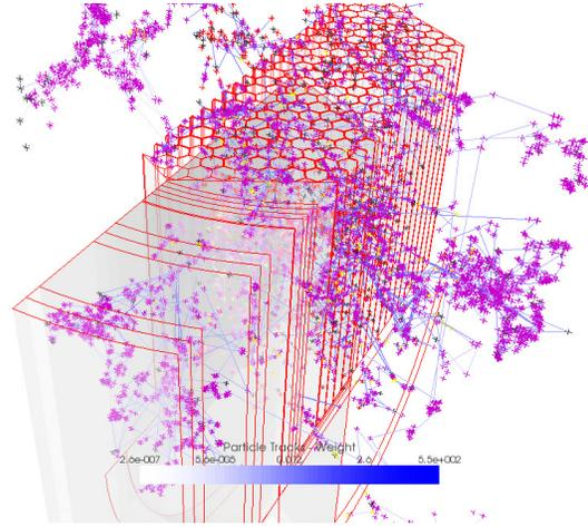
Figure 3. History log coloured by event weight on translucent wire frame of reactor with geometry cut away.
