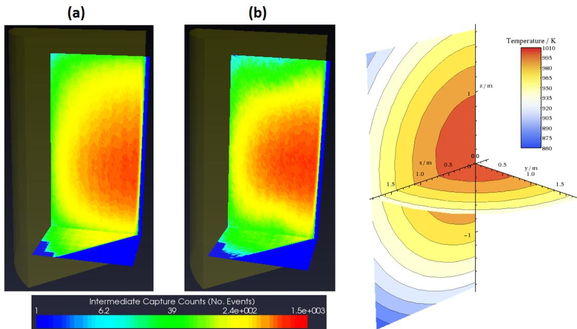
**Figure 5: Axial and radial averages of intermediate capture events across the Hoogenboom and Martin benchmark 1/8<sup>th</sup> core model; (a) fixed temperatures and (b) estimated temperature profile. Estimated temperature profile across the core in the axial and radial directions is shown far right.**
