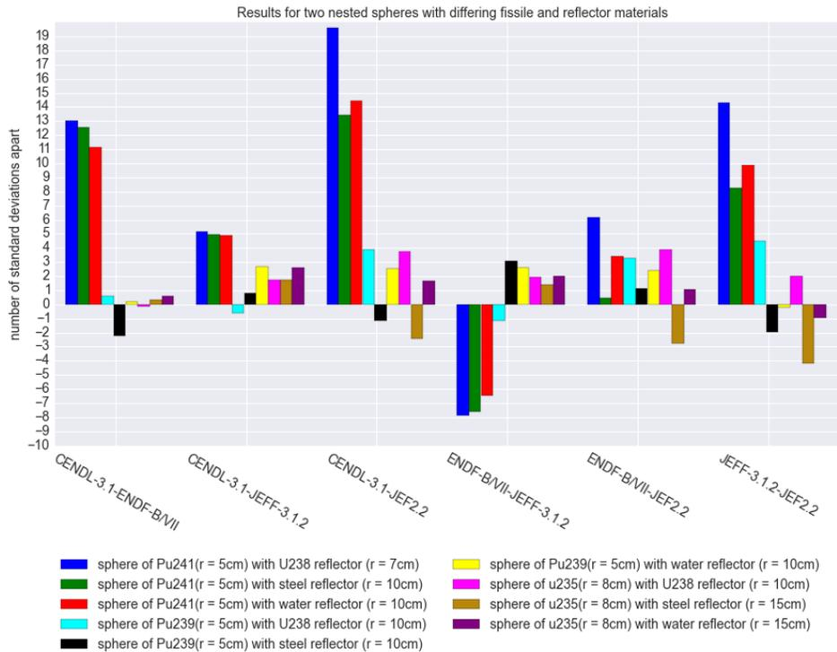
**Figure 4: Nuclear data library comparison using nested spheres model with varying combinations of  $^{239}\text{Pu}$ ,  $^{241}\text{Pu}$  and  $^{235}\text{U}$  fissile material with  $^{238}\text{U}$ , water and steel reflectors.**
