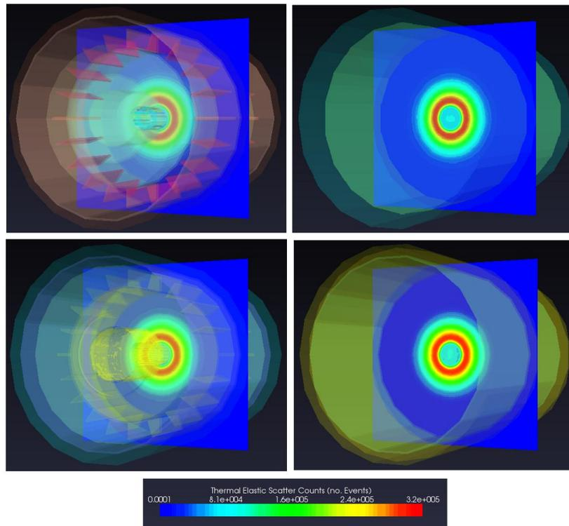
**Figure 3: Thermal elastic scatter events for the transport flask model using geometries; (top-left) FG, (top-right) IGES body, (bottom-left) POLY body and (bottom-right) TETMESH Hole.**
