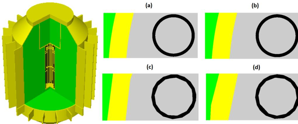
**Figure 1: Transport flask model: (far left) Cut away 3D ray-trace image of entire geometry with fuel rods, stainless steel structure and water tank shown in black, yellow and green respectively. Detail 2D ray-trace images in the axial plane: (a) FG, (b) IGES body, (c) POLY body and (d) TETMESH Hole.**
