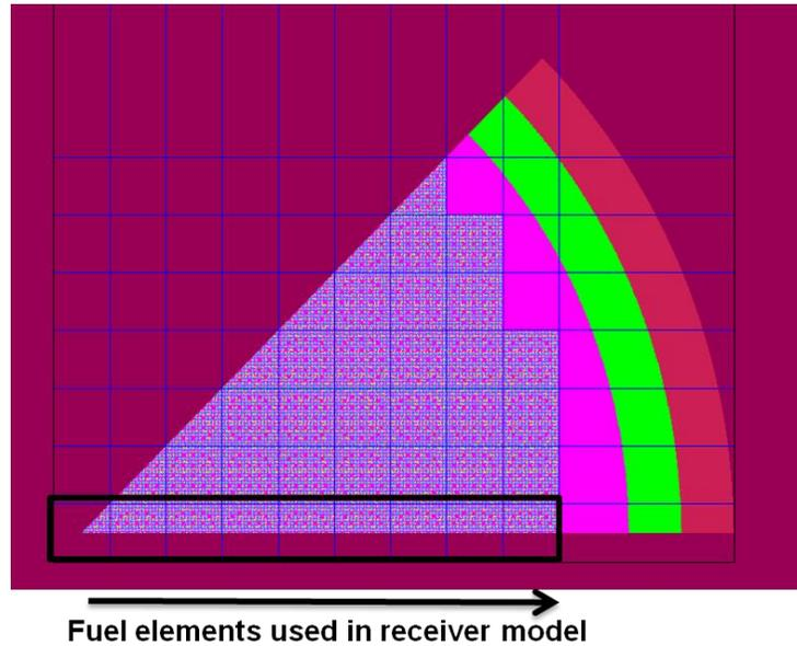
**Figure 3** Burn-up mesh superimposed on PWR model showing the range of axial fuel elements that are considered as part of the spatially-dependent burn-up study
