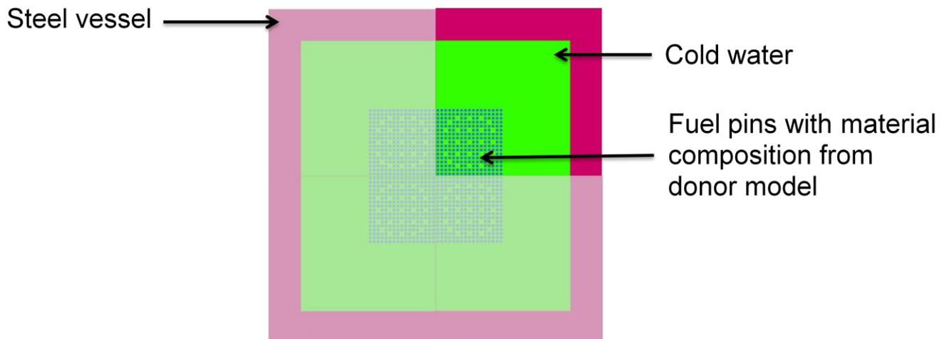
**Figure 2 Receiver model for BUC analysis.**
