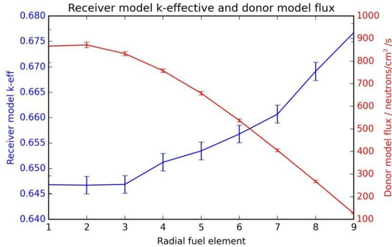
Figure 5 Variation in receiver model k-effective with changing radial fuel element, showing one group flux averaged axially over the fuel element. Errors are 3 standard deviations.
