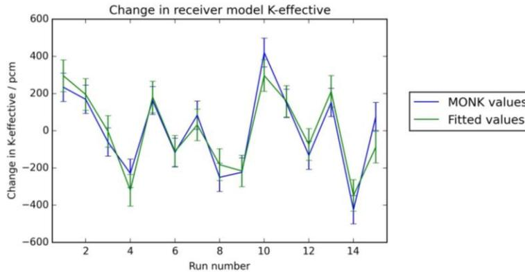
**Figure 10 Change in k-effective of receiver model for each run showing validity of linear fit**
