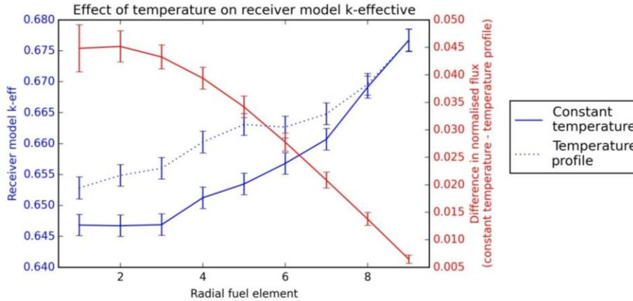
Figure 8 Effect of applying a realistic temperature profile on k-effective for the receiver model
