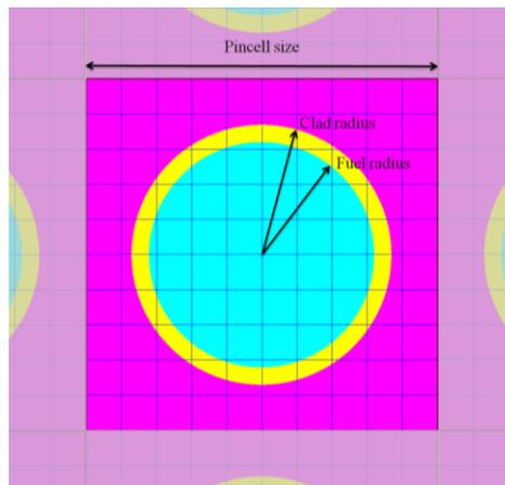
Figure 9 Infinite array of fuel pins showing geometric properties varied in uncertainty study
