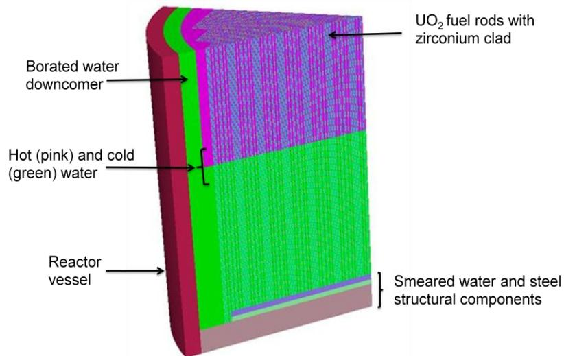
Figure 1 Visual Workshop image of 1/8<sup>th</sup> core PWR model based on the Hoogenboom and Martin benchmark.
