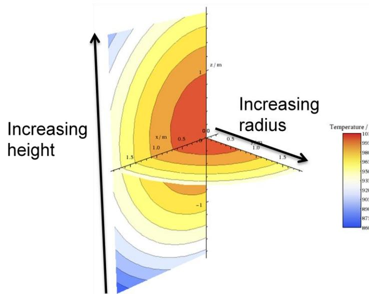
Figure 6 Fuel temperature profile showing axial and radial variation in temperature!
