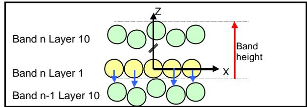
Fig. 9 Mode 3 packing – sphere relocation
