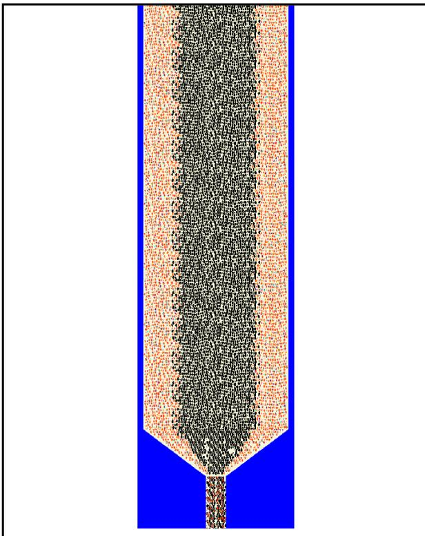
**Fig. 3** PBMR hole packing spheres into a reactor core.
