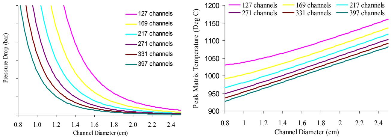
**Core Pressure Drop and Peak Matrix Temperature for the Plate Sub-Assembly Geometry**
