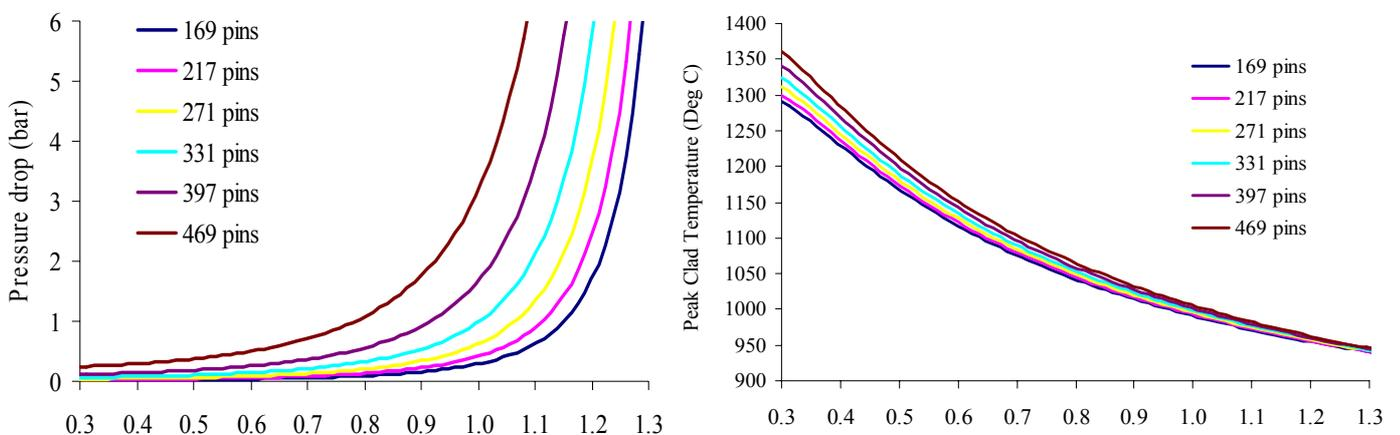
**Core Pressure Drop and Peak Matrix Temperature for the Block Sub-Assembly Geometry**
