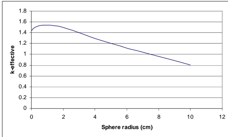
**Figure 4. Variation of  $k_{\text{effective}}$  with mixing.**
