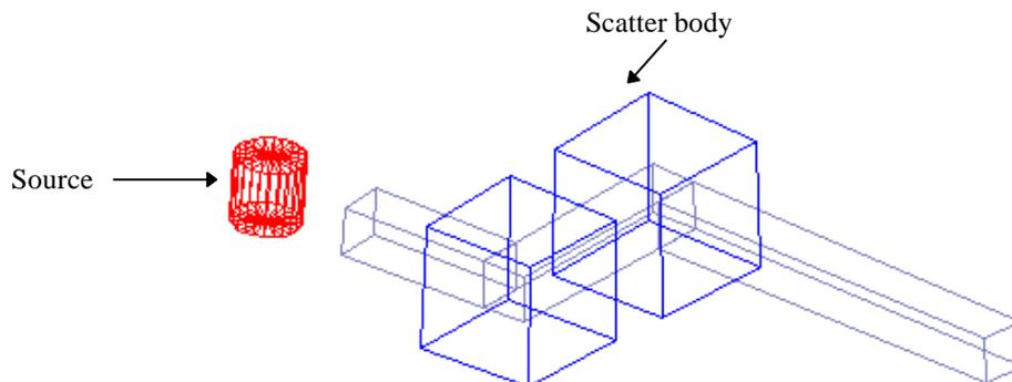
**Figure 8 - VISTA-WIRE Representation of a Multi-legged Duct**
