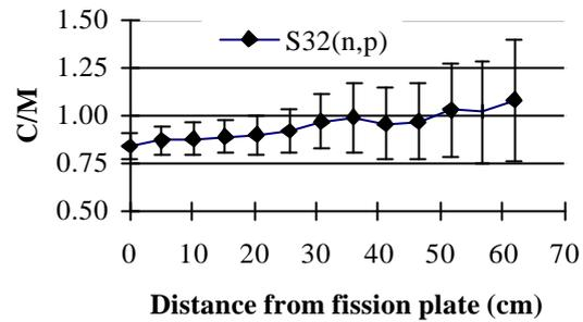
Fig. 6 C/M for  $\text{S}^{32}(\text{n},\text{p})$  in the Iron Benchmark
