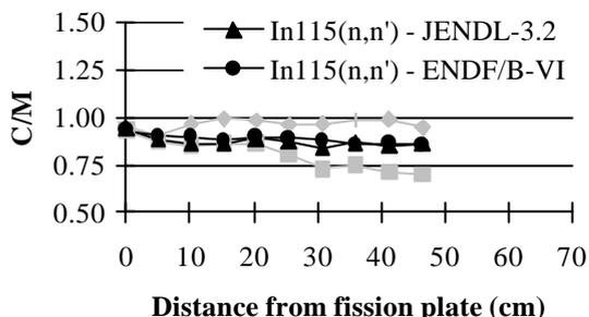
**Fig. 4** C/M for  $In^{115}(n,n')$  in the Iron Benchmark using JENDL-3.2 and ENDF/B-VI data
