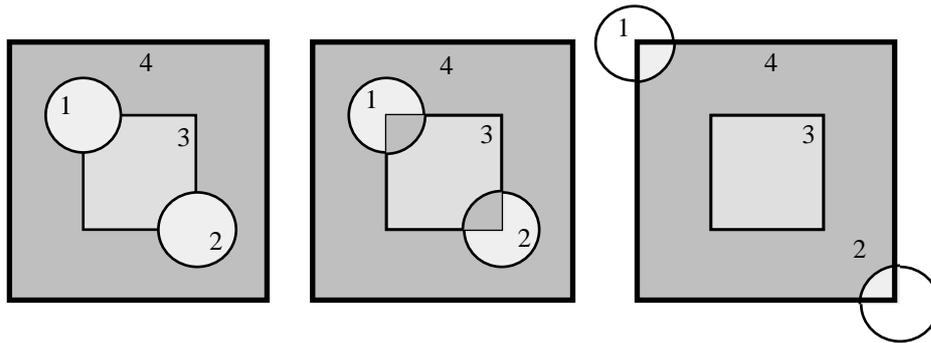
In a general part the container does not necessarily have to be the last body specified and the order of specifying bodies and zone definitions is at the user's discretion. Note that the order of presentation does however serve to number the bodies and similarly for the zones independently of the bodies.
