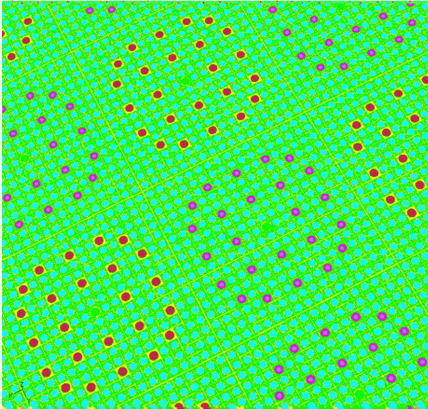
**Figure 3. Core layout showing elements with RCCA, GRAY control rod assemblies and fuel assemblies with burnable absorber**
