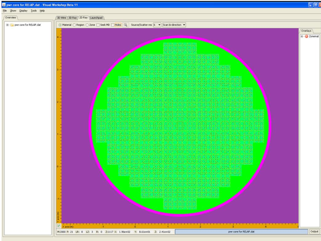
Figure 1. PWR Model Whole Core layout
