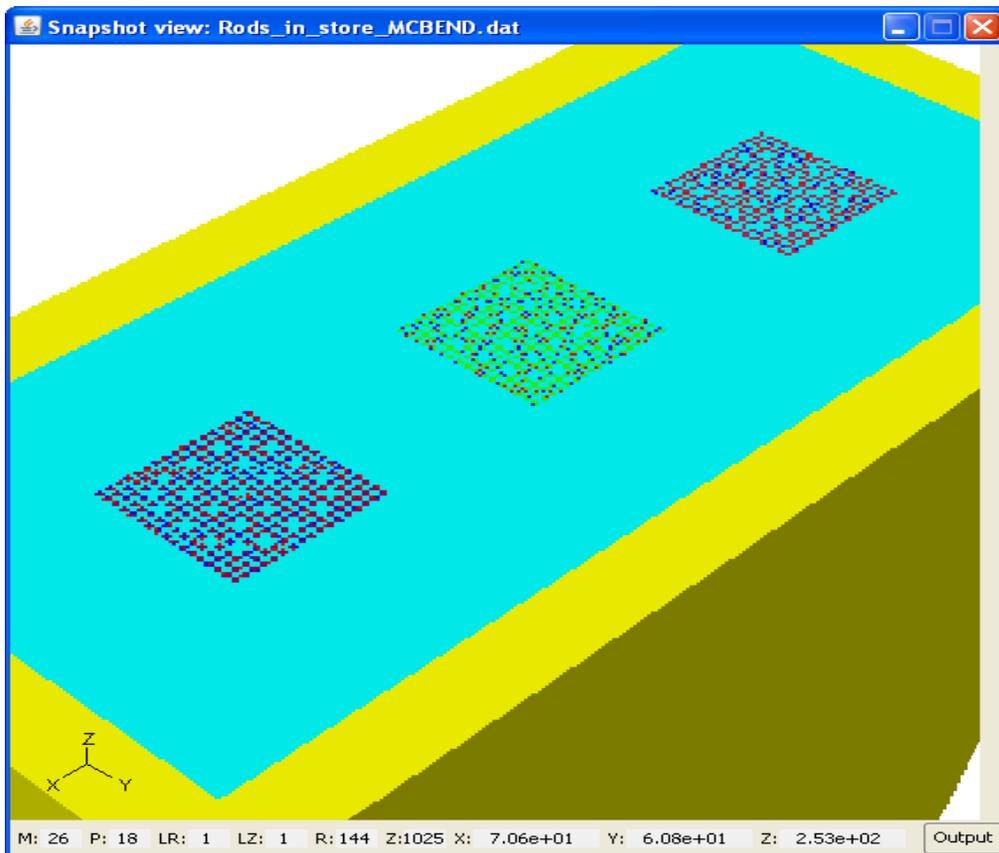
Figure 5. Showing 3 fuel elements in water through a z-slice view
