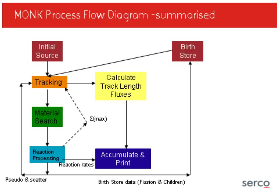
Figure 11. MONK Process flow diagram
