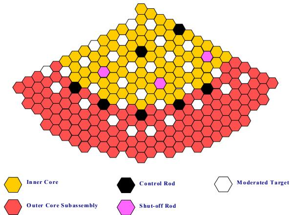
Figure 3 : Core Layout with In-Core Moderated Targets
