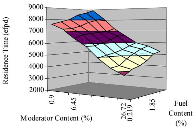
Figure 10 : Residence Time Required to Reach 90% Mass Destruction for In-Core Moderated Targets
