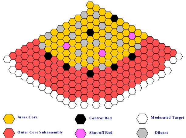
Figure 4 : Core Layout with Ex-Core Moderated Targets
