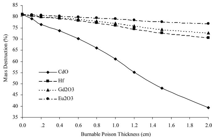
Figure 7 : Mass Destruction for In-Core Targets with ZrH<sub>1.65</sub> Moderator
