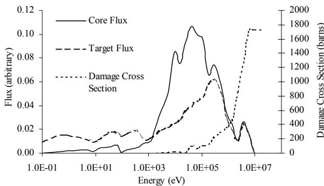
Figure 5 : Neutron Energy Spectrum and Clad Damage Cross Section for In-Core Moderated Targets
