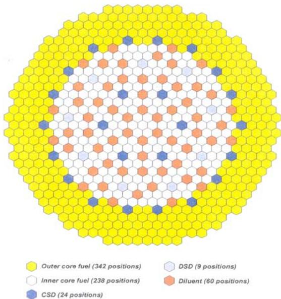
Figure 1. Gas Cooled Fast Reactor Core layout
