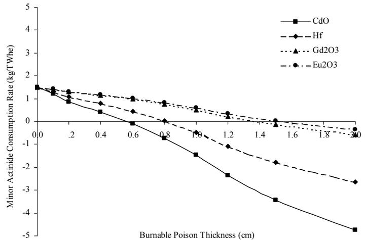
Figure 8 : Net Minor Actinide Consumption for In-Core Targets with ZrH<sub>1.65</sub> Moderator
