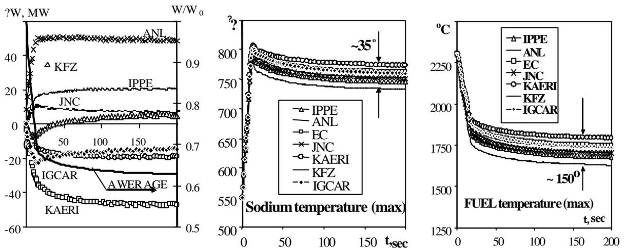
Fig. 11. Change of power and basic temperatures in ULOF accident
