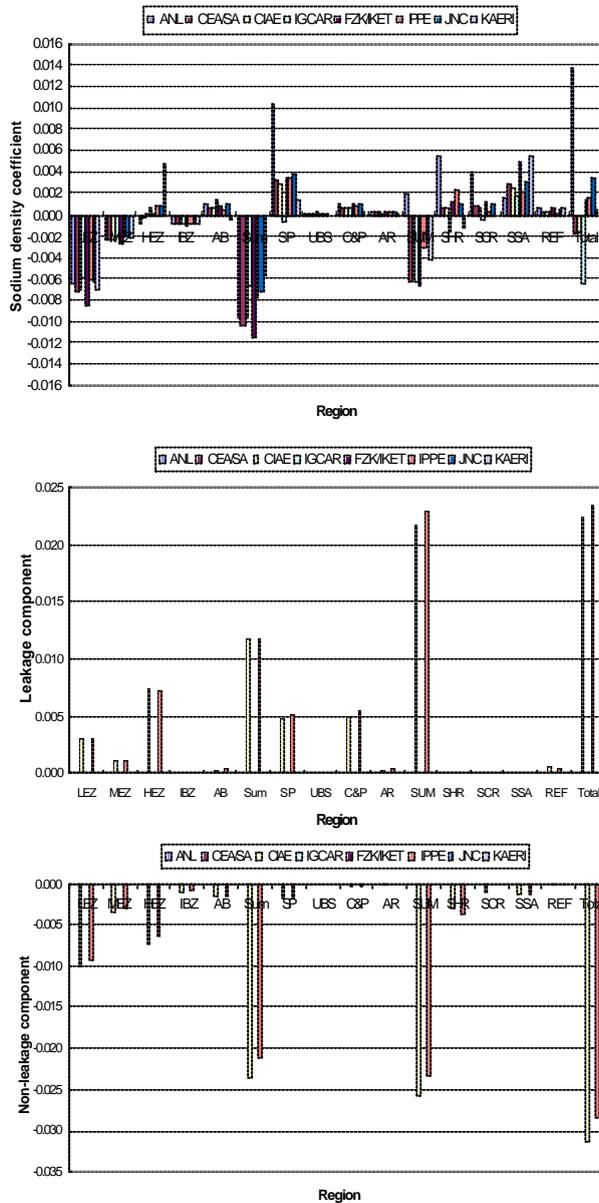
**Fig. 5.** Regionwise sodium density coefficients
